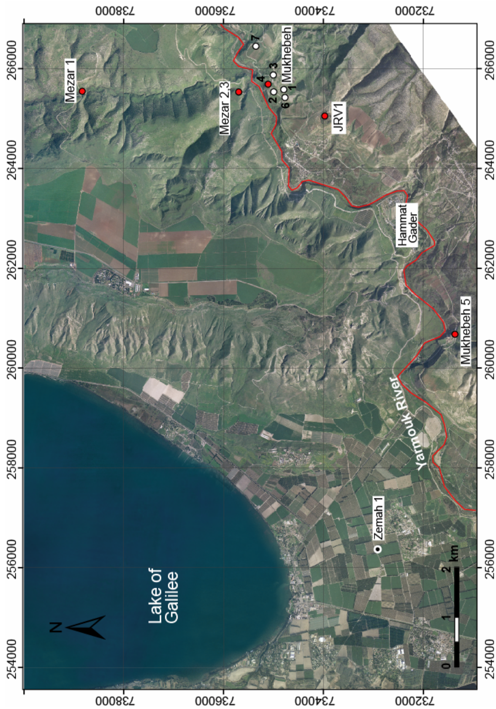
Figure 8: Location of the geothermal system east of the Sea of Galilee. Red circles represent boreholes tapping the Judean aquifer and white circles represent boreholes tapping shallower aquifers. The deep Zemah 1 borehole (4250 m) is drilled into the basin fill.
