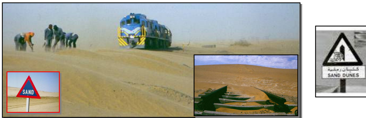
Figure 1.2 Examples of damage from sand and dune mobilization in Africa.
