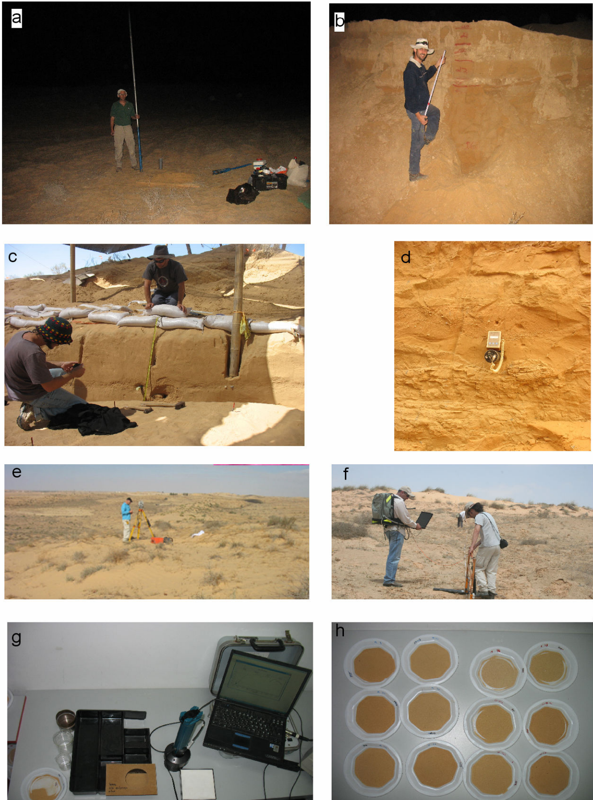
Figure 2.5 OSL and GPR field work methods and spectroscopic measurement setup. a. OSL sample extraction by dune-drilling and from an exposed section (b) at night. c. OSL sampling at the Sekher VI section with plastic tubes. d. Cosmic and gamma dose rate measurement with a calibrated portable Rotem P-11 gamma scintillator. e. Topographic surveying with a Total Station, here positioned upon the BM transverse dune. f. GPR profiling at the BM site. g. Spectroscopic measurement set up including a (1) black box for the sample and (2) probe muzzle. h. Different redness intensities of sand samples being room-dried in plastic plates.
