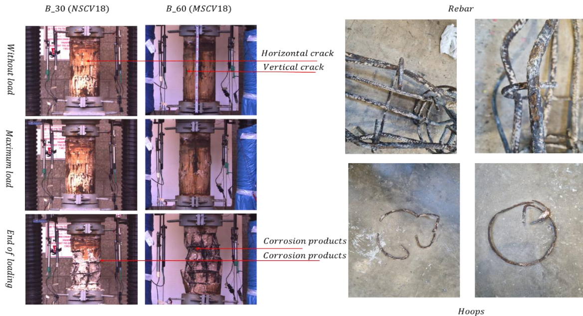
Figure 11: Samples exposed to a voltage of 18 volts in a salt solution for a period of 28 days and bearing capacity
