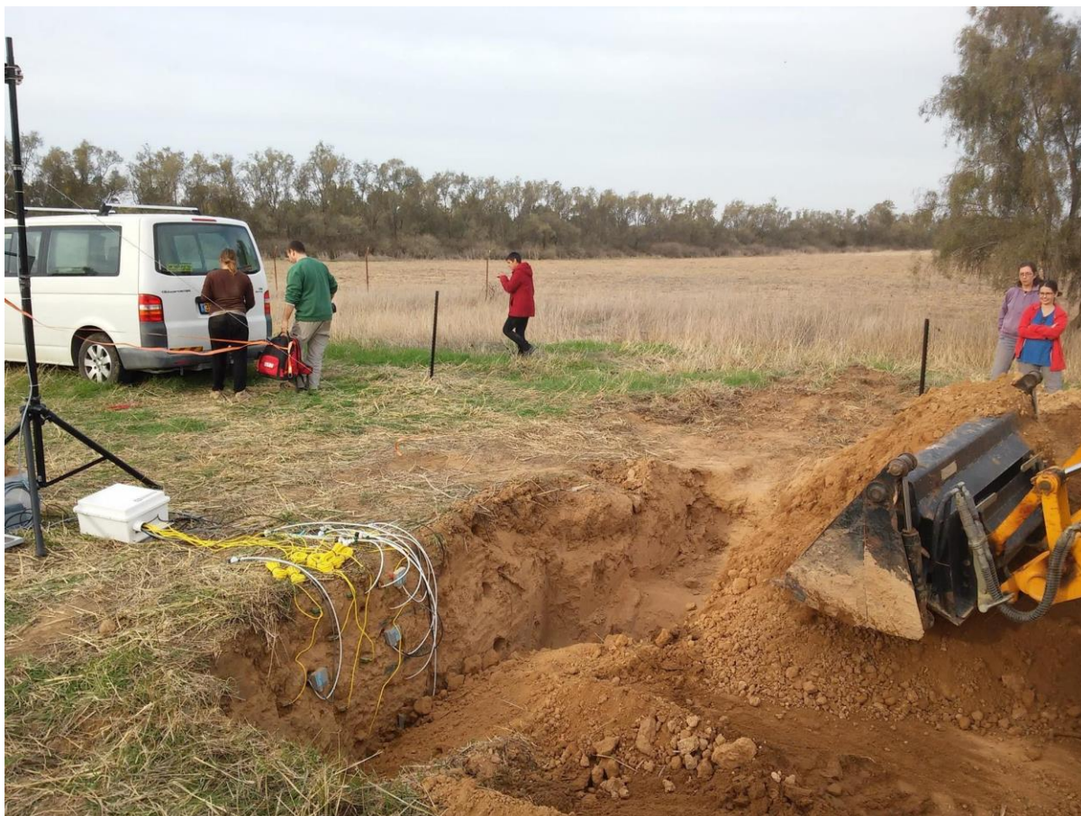
Appendix ii-2 Monitoring station in Gilat: sensors installed into the undisturbed trench wall. Mud inserted the TDR .sensors for continuity of soil. Than the trench was covered. Grassy surface
