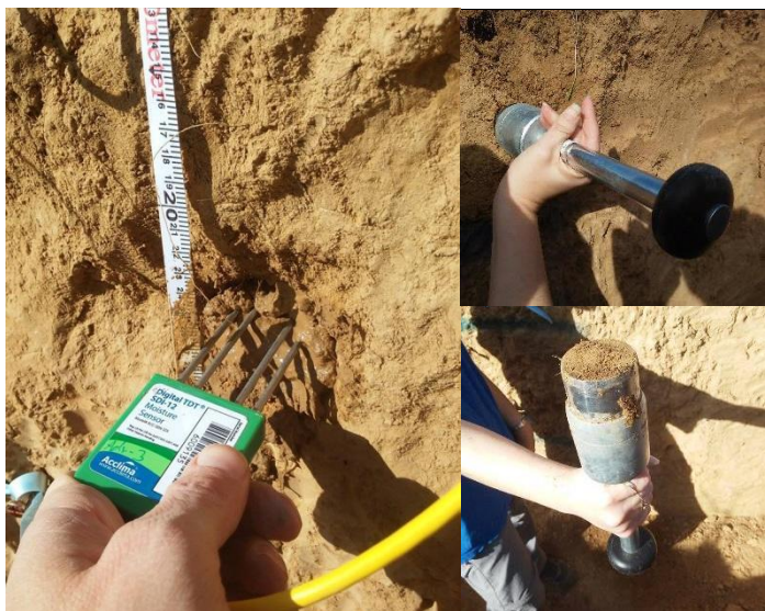
Appendix ii-3 on the left: TDR installation with mud filling the space around the sensor. On the right: the in-situ soil .sampler
