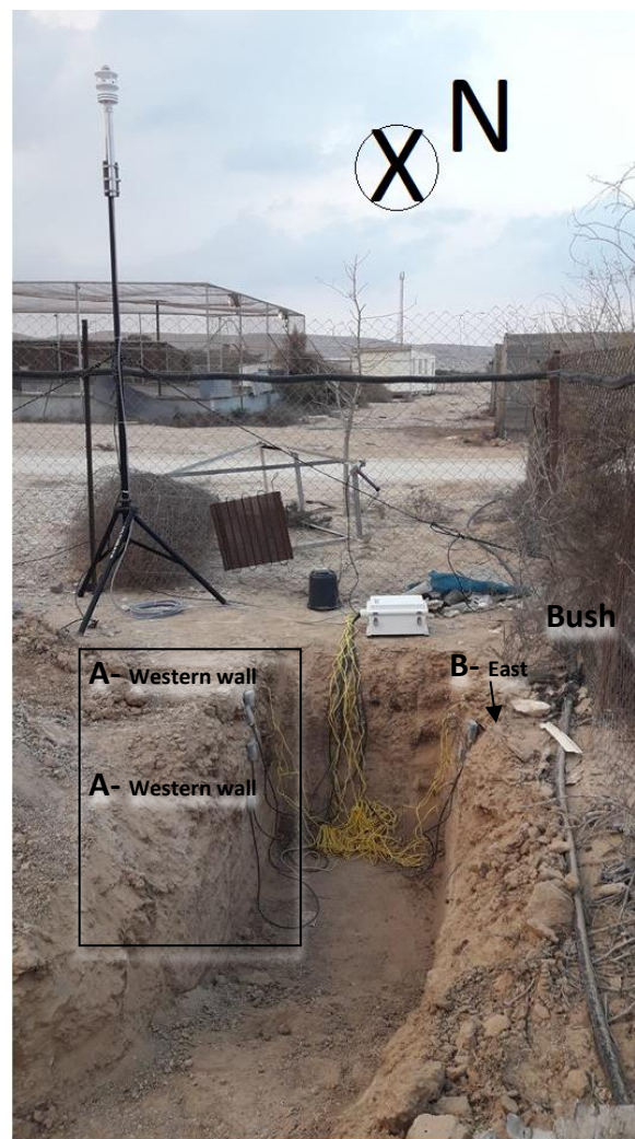
Appendix iii-2 Soil profile of Sde Boker monitoring station. Open trench, view direction: North. Sensors were installed into the undisturbed soil in the western wall (A), under bare soil, under the bush, and into the undisturbed soil in the eastern wall (B) under bare soil.
