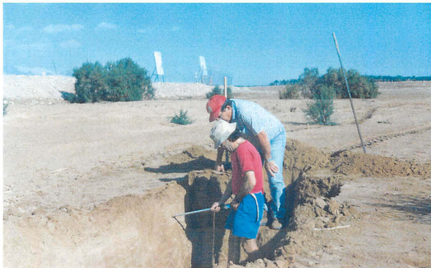
Figure 6.10. Engineering tests using a Penetrometer, within the trenches at site C, Eilat.
