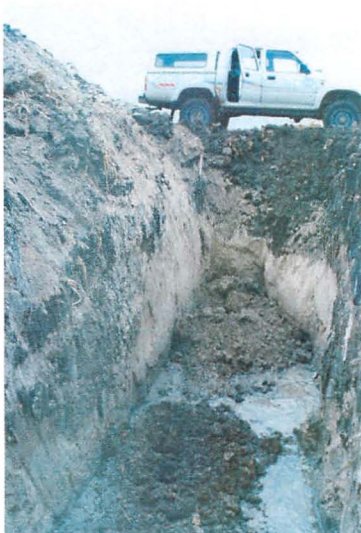
Figure 6.13. Ein HaMifratz Northeastern trench. The groundwater level is here at depth of 3 m.
