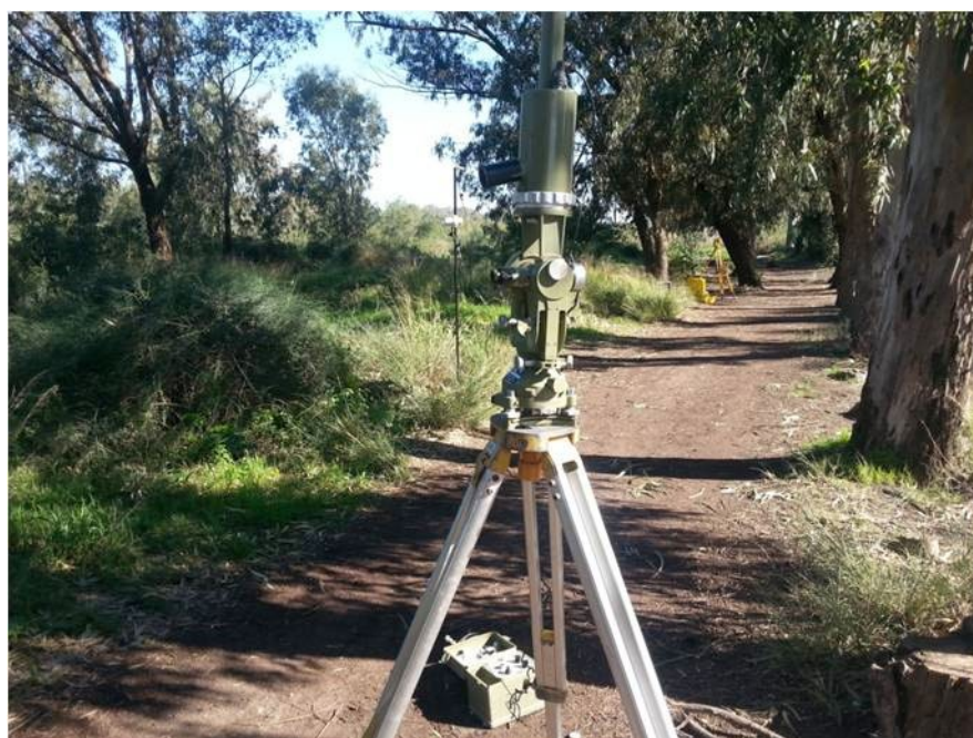
Fig.13 Instruments for the vector of magnetic field measuring at the one of the point of the network ("River Alexander"). In the foreground: the Wild Gyro instrument GAK1 mounted on the Wild T2 theodolite, in the background, at the left: proton magnetometer sensor GSM19; at the right: theodolite DIM.
