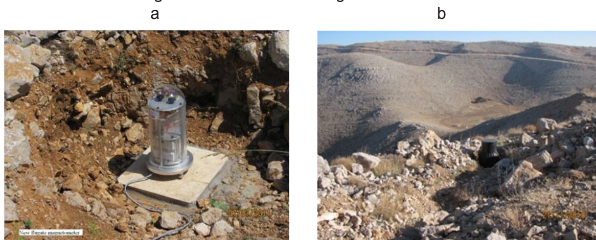
Fig. 8a, b: FGE fluxgate magnetometer installed at the Hermon site
