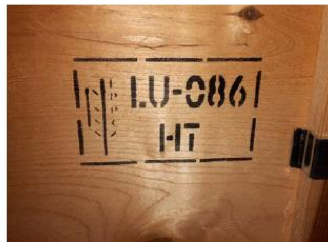
Vertical line to right of symbol is missing
