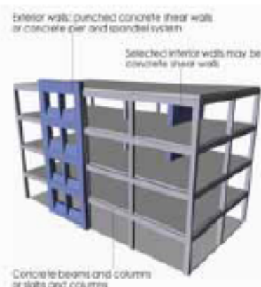
C2f: Concrete Shear Walls (Gravity Frame Systems)
