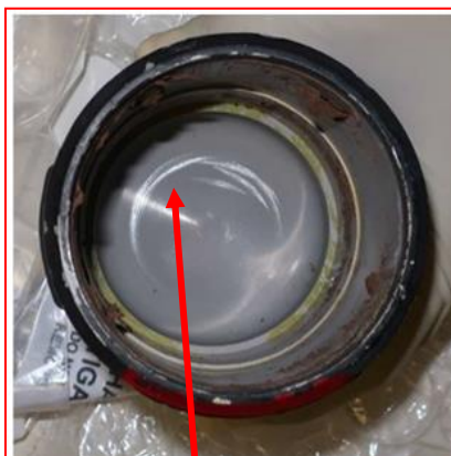
Interior of red damper housing With semi-circular witness marks
