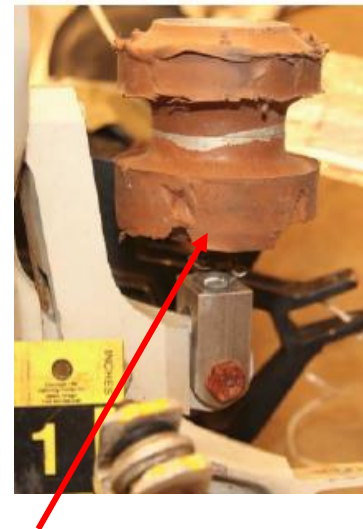
The fatigued elastomeric material
