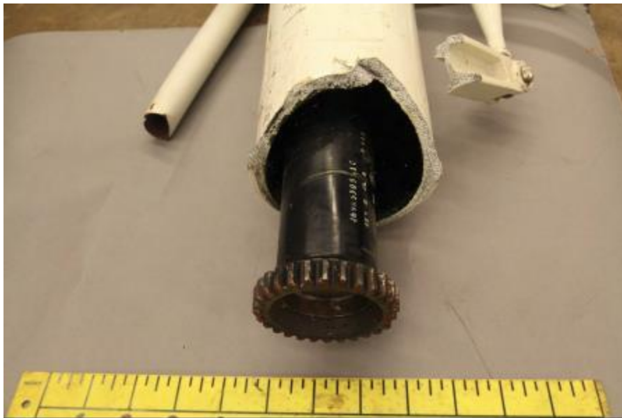
Figure 4 – The fracture surface of the main rotor mast, viewed from an oblique angle
