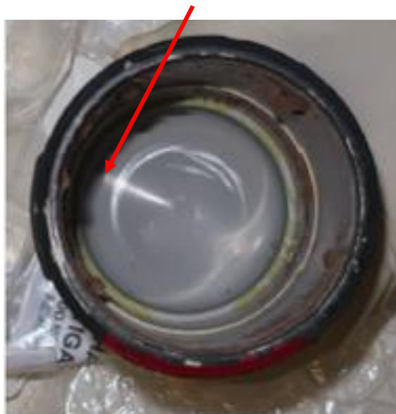
Figure 4- Interior of red damper housing showing semicircular witness marks.
