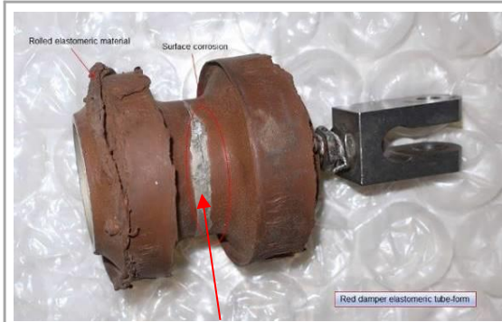
Figure 2 - Red damper tube form. Corrosion at seam between disks
