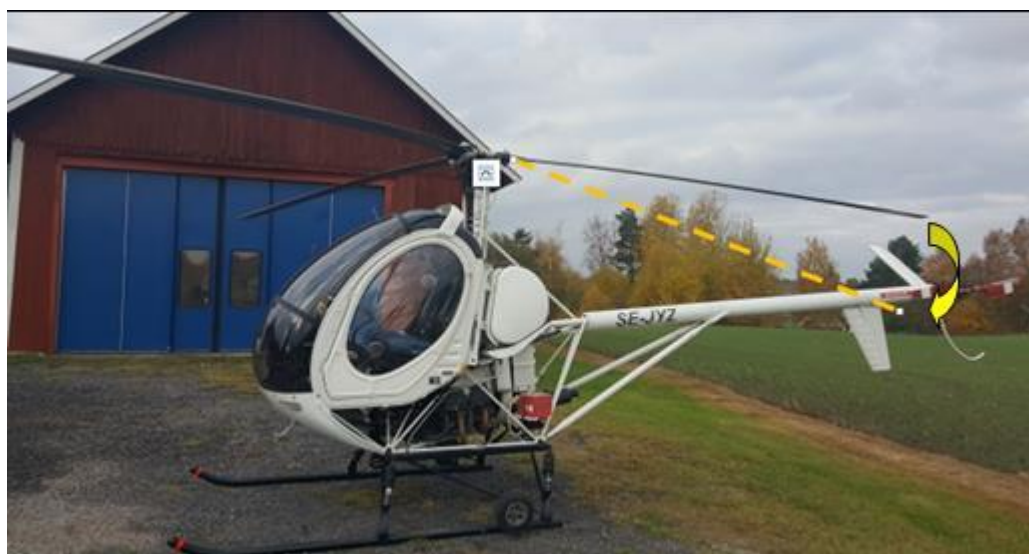
Accident helicopter under Swedish registration. Dashed line indicates the blade sag which will hit the boom
