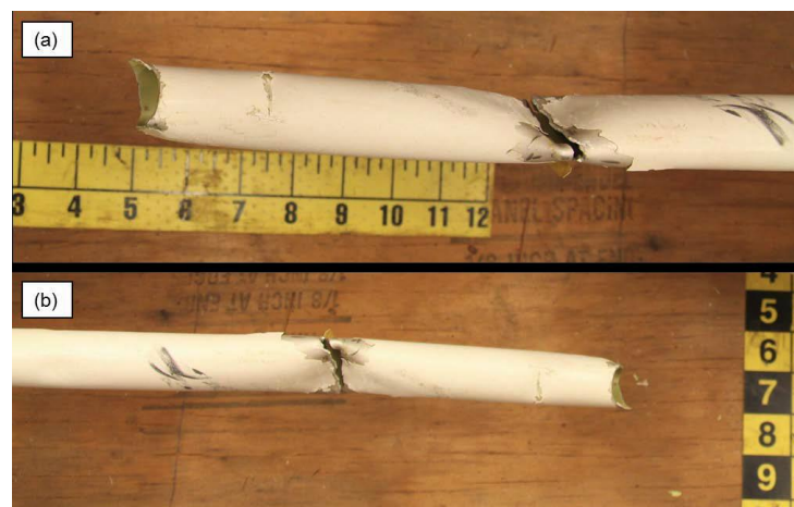
Figure 2 – One of the fractured pitch change links, as received
