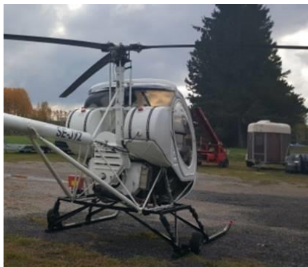
Image of the accident helicopter, still under Swedish registration, the cross bar is straight
