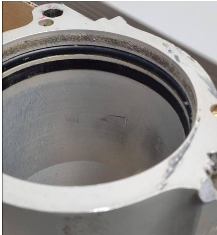
Figure 16 - Imprint marks on the piston
