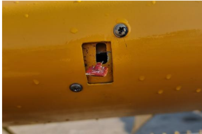
Figure 7 - Angle of Attack Sensor
