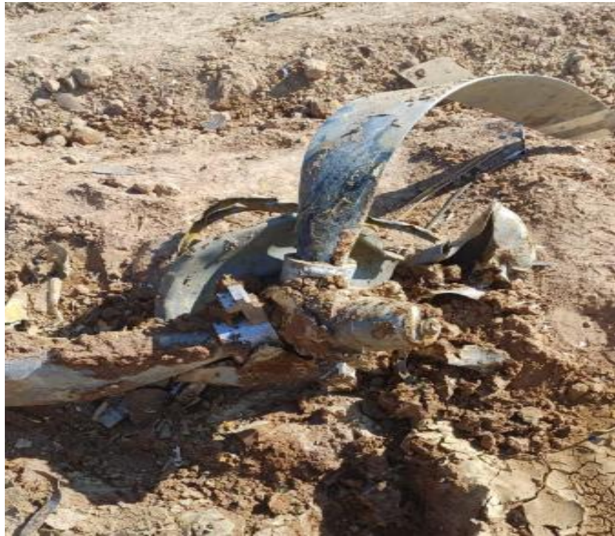
Figure 3 - Propeller - pitch mechanism and blades
