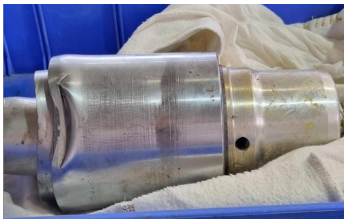
Figure 15 - Imprint marks on the cylinder
