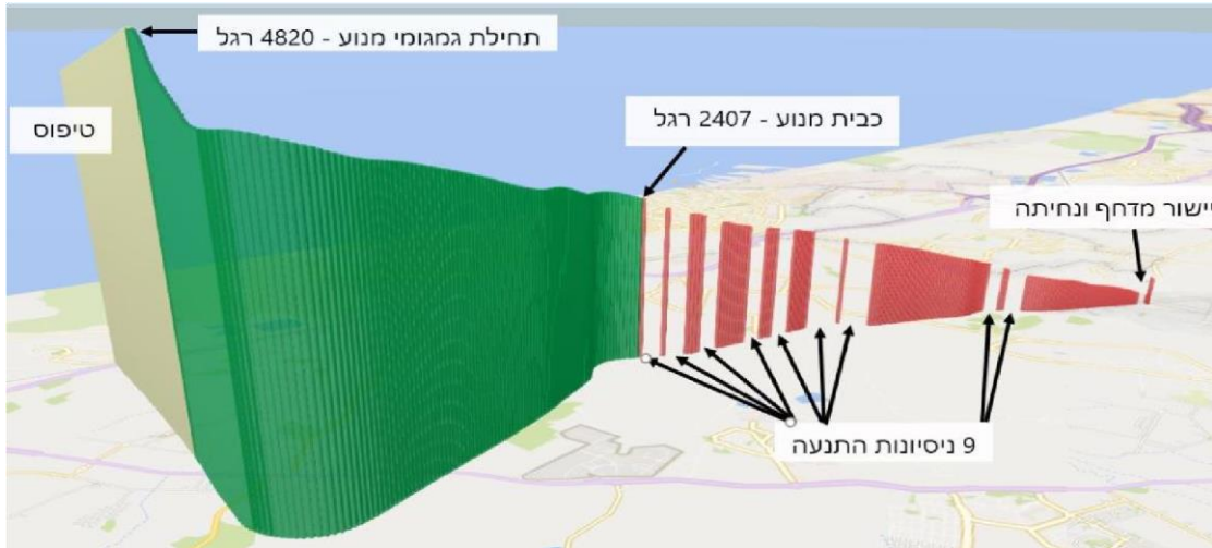
Figure 4 - Flight Profile and Start Attempts Characterized by Loss of GARMIN Data (Electrical) During Use of Starter
