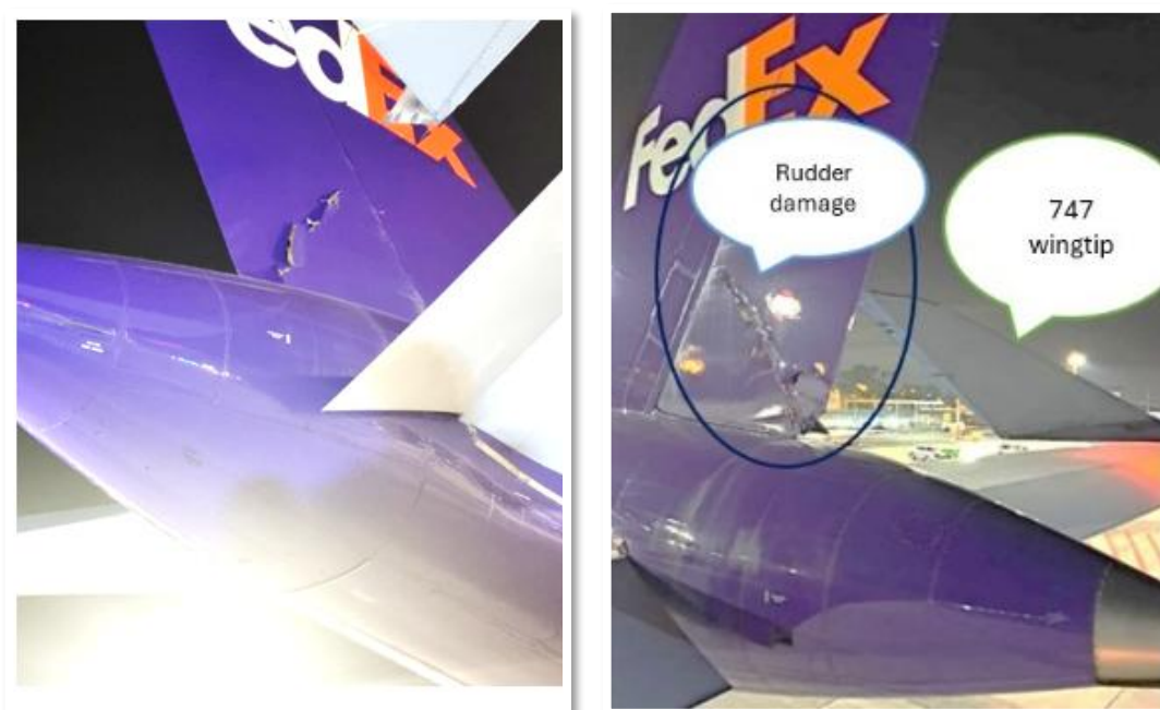
Figure 2 - Rudder of the 757-200F, wingtip of the 747, and impact marks
