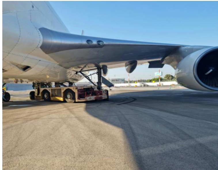
Figure 8 - Tug position and tire marks
