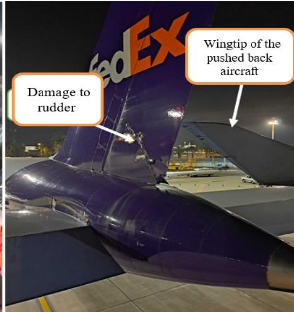
Rudder damage of the parked FedEx aircraft
