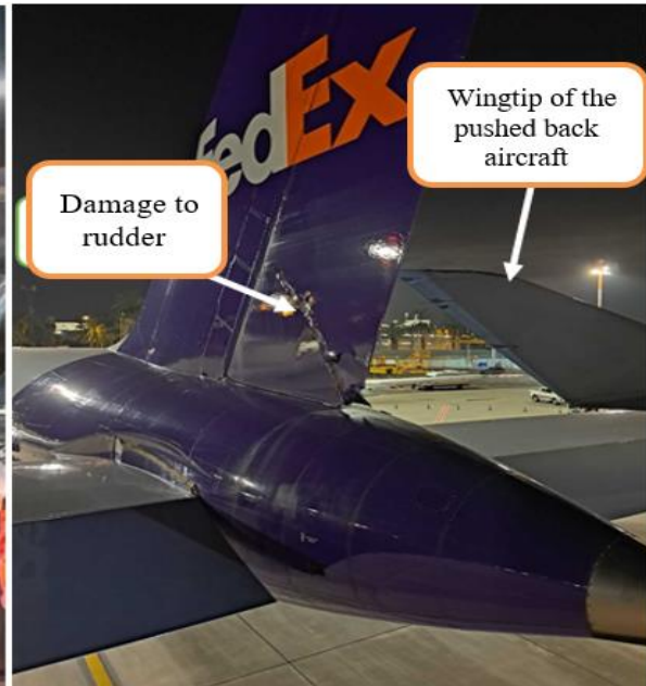
Rudder damage of the parked FedEx aircraft
