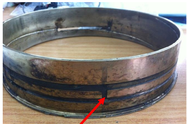
Blocked Grease Groove
