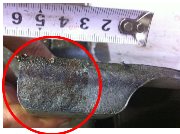
Surface of the crack
