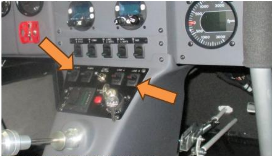
Figure-1 : example of configuration with safety guards missing
