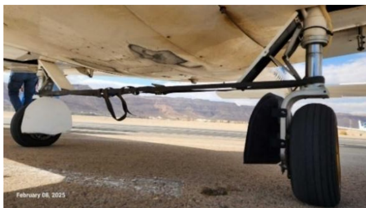
Picture 4 - Securing the landing gear using tie-down straps and a ratchet
