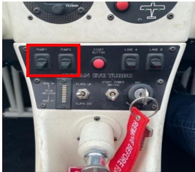
Picture 6 – Location of the fuel pump switches on the aircraft center console
