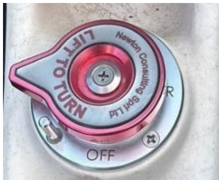
Picture 5 - Fuel tank selector position as found after the accident
